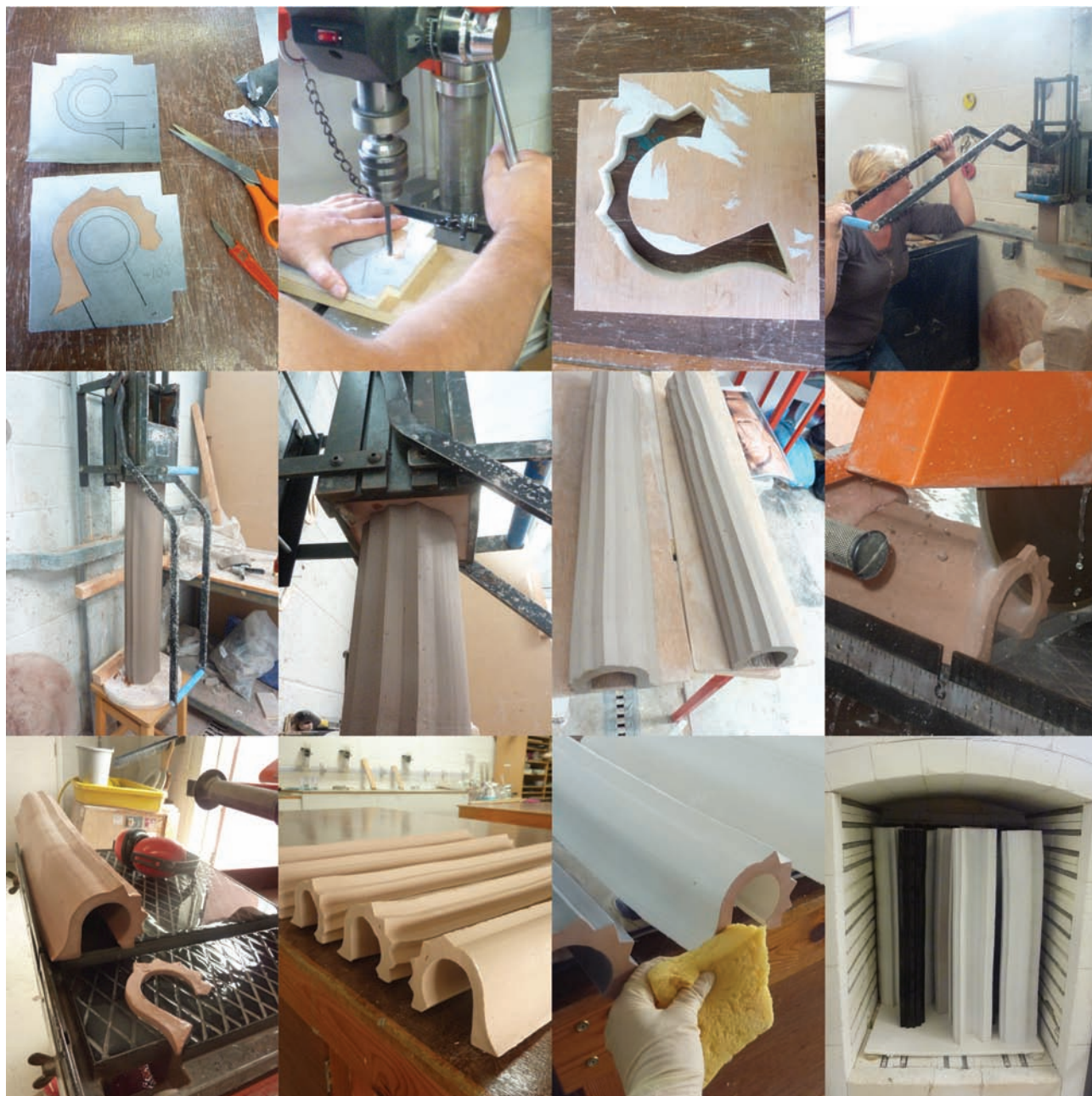
Production process of the Prismatic-Rod Screen ceramic components. © Wendy Lawrence.
