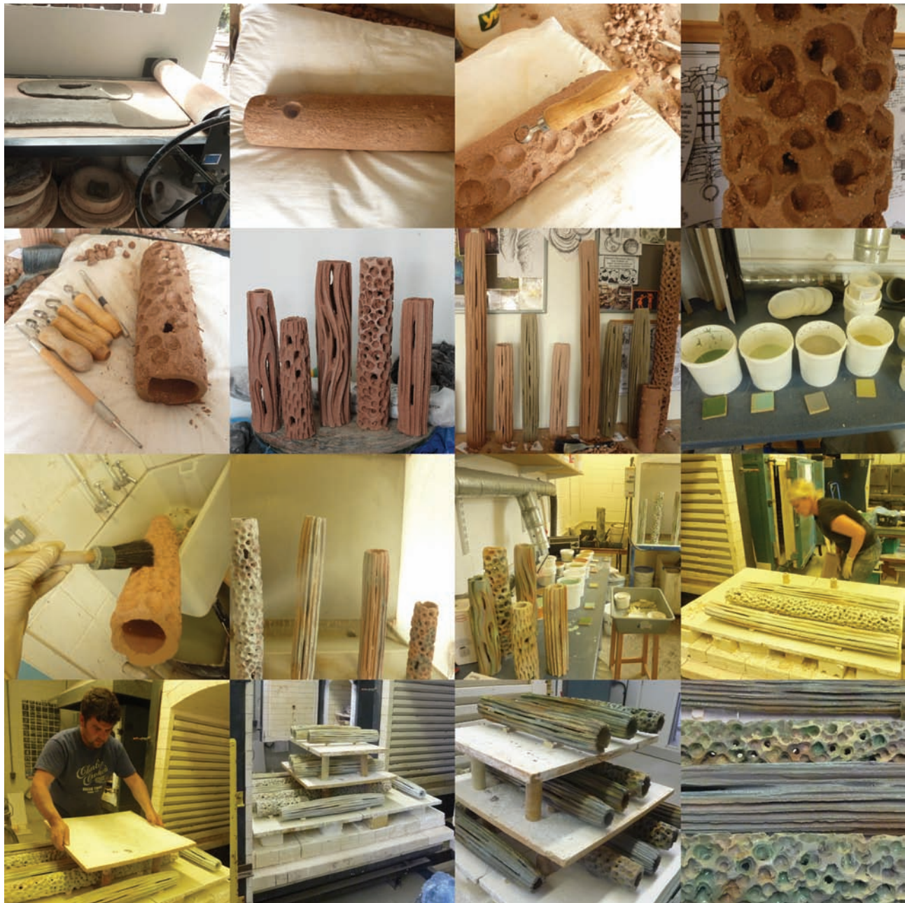
Production process of the Hydroponic Chandelier ceramic components. © Wendy Lawrence.
