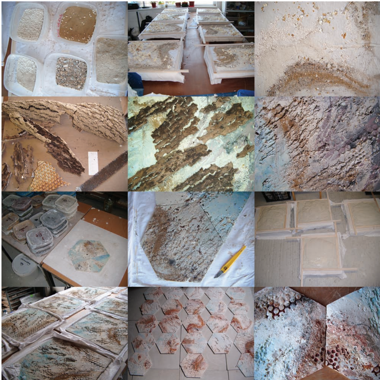
Production process of the Tessellating Hexagonal Curtain ceramic components. © Jenny Beavan.
