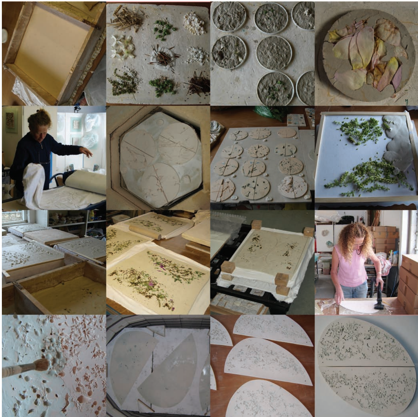
Production process of the Dynamic Ceramic Ceiling ceramic components. © Jenny Beavan.
