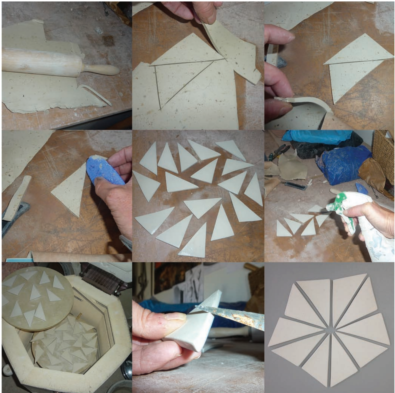
Production process of the Performative Ceramic Surface ceramic components. © Wendy Lawrence.
